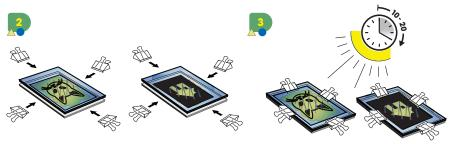
Use the **provided clips** to pinch the contact-printing frame tight.
