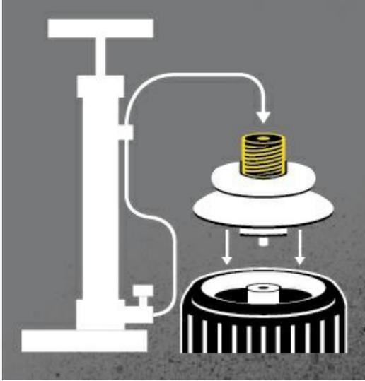
*Pump used with Adapt-AIR coupling*
